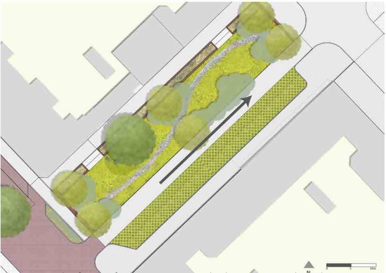
Figure 66 Masterplan of one unit of Copernicusstraat. Two way drive becomes one way. A dry wandering stone stream across the green area. Constructed rain garden box with Amsterdam School detailing become the edge
