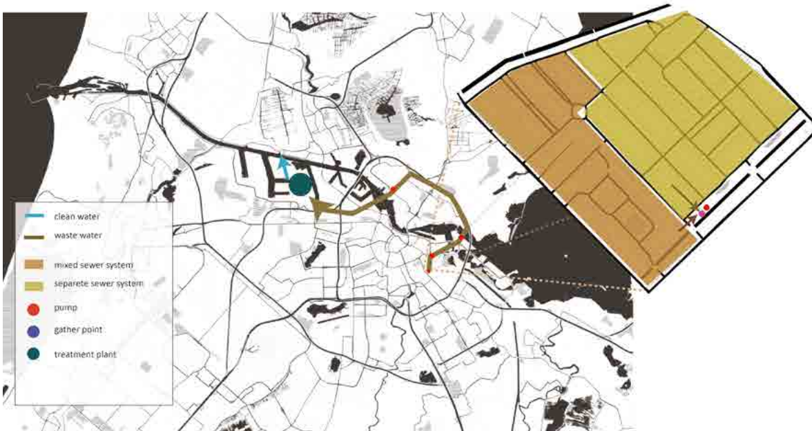
Figure 29 The waste water sewage system on city and neighbourhood level, the waste water will be collected in the pump station in Galilei Park and transport to treatment plant
