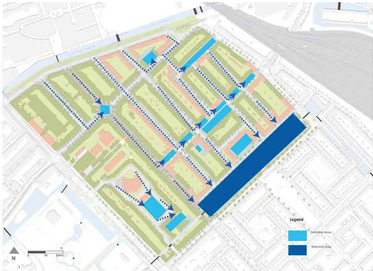
Figure 52 Surface Water system on neighborhood level. Galilei Park as primary retention area, and Copernicusstraat is the secondary
