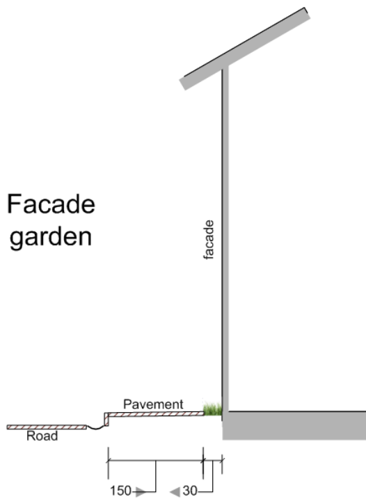
Figure 9: Design criteria of a facade garden
